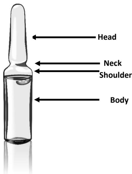
**Figure 3: Parts of an Ampule**
